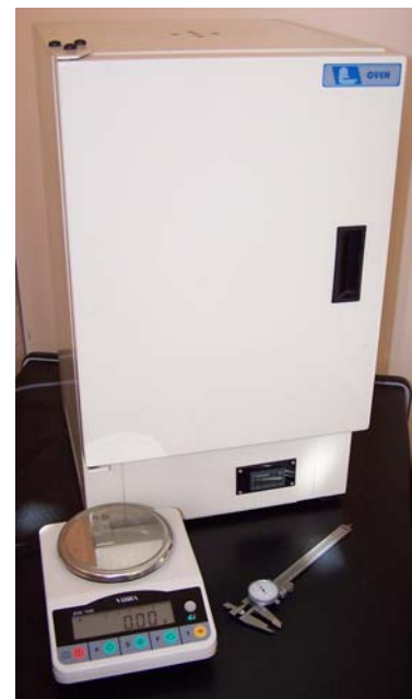
Oven dry testing – Provides the most accurate moisture content test.
