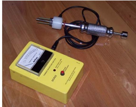
Resistance moisture meter - Measures moisture content between the pins – Need to correct reading for temperature and species.
