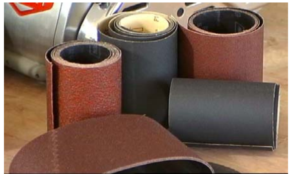
During the sanding process progressively finer papers are used.
