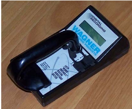
Capacitance moisture meter - Measures average moisture content – Need to set species density.
